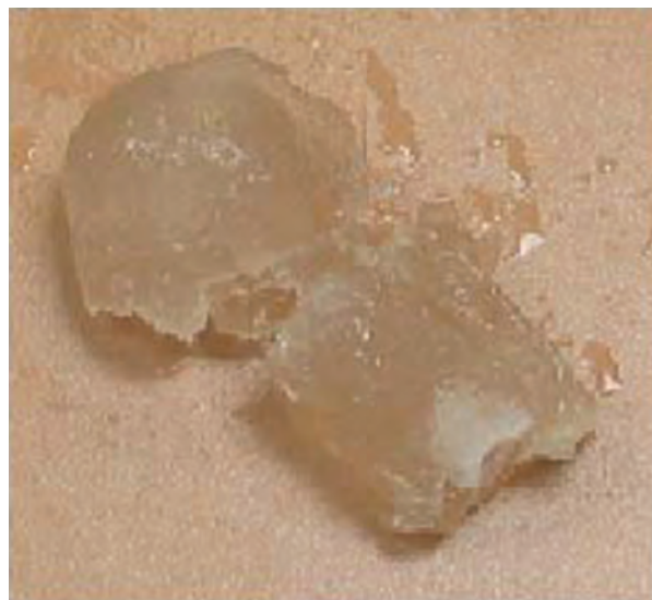
Figure 7 SPH platform recovered from gastric simulator.
